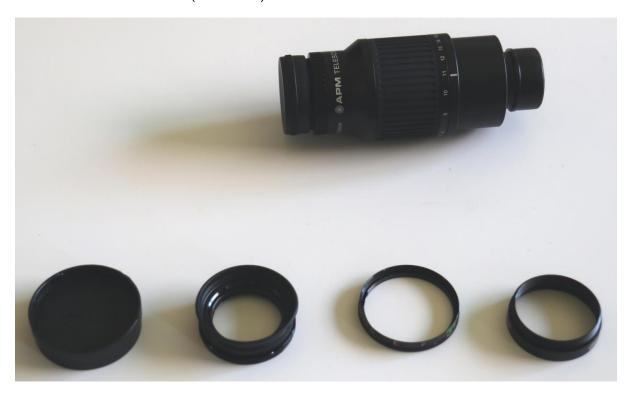
Separate the Dioptrx to give the lens ring and the engraved (green) ring. Loosely fit the engraved Dioptrx ring over the male thread on the M43 extension:
